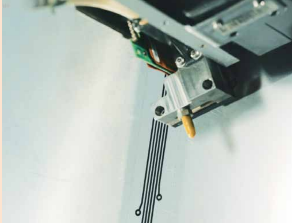
Manufacture of printed wiring harness segment on the inside of a vehicle door via 6-axis robotic-controlled inkjet printing technology.
