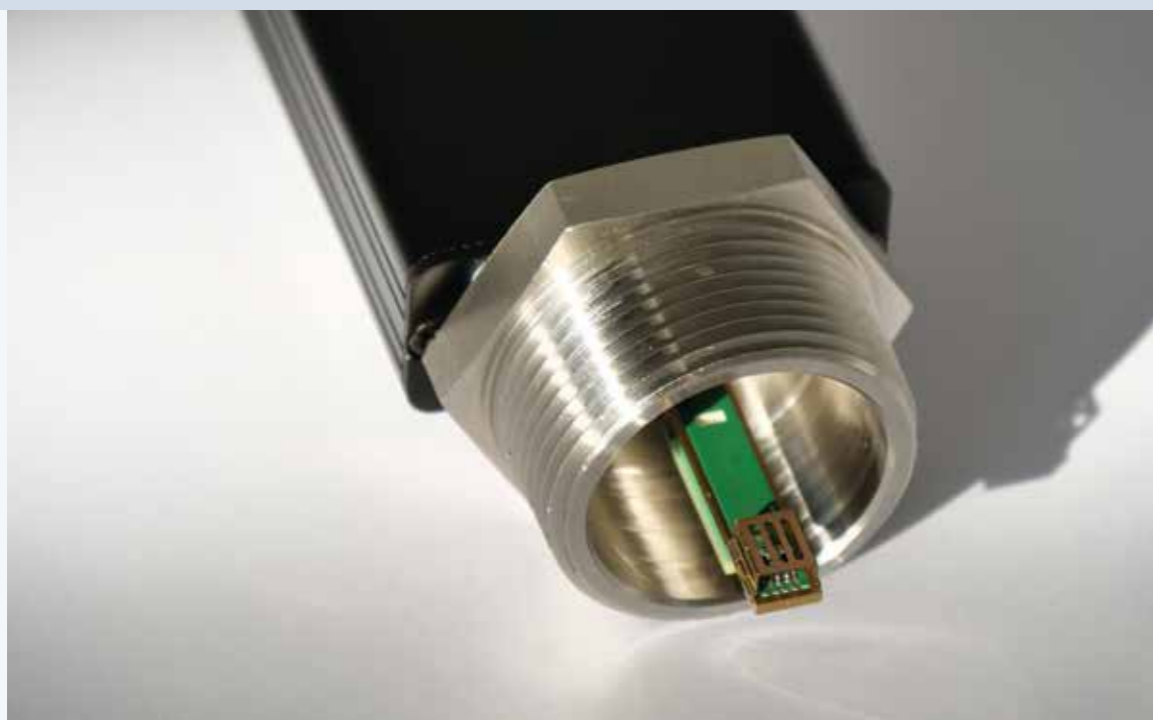
Detailed view onto the immersed part of the viscosity and density sensor.
