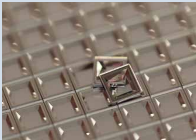
CuO/Al bonded Si-quartz glass demonstrator for optical components.
